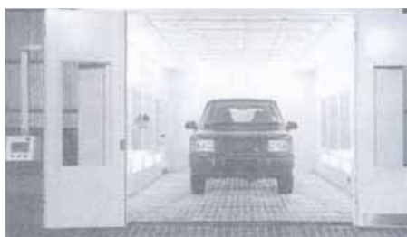
Figure 4 Typical spray booth for vehicles
