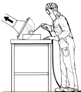
LEV used to help draw welding fume from the breathing zone of a welder
