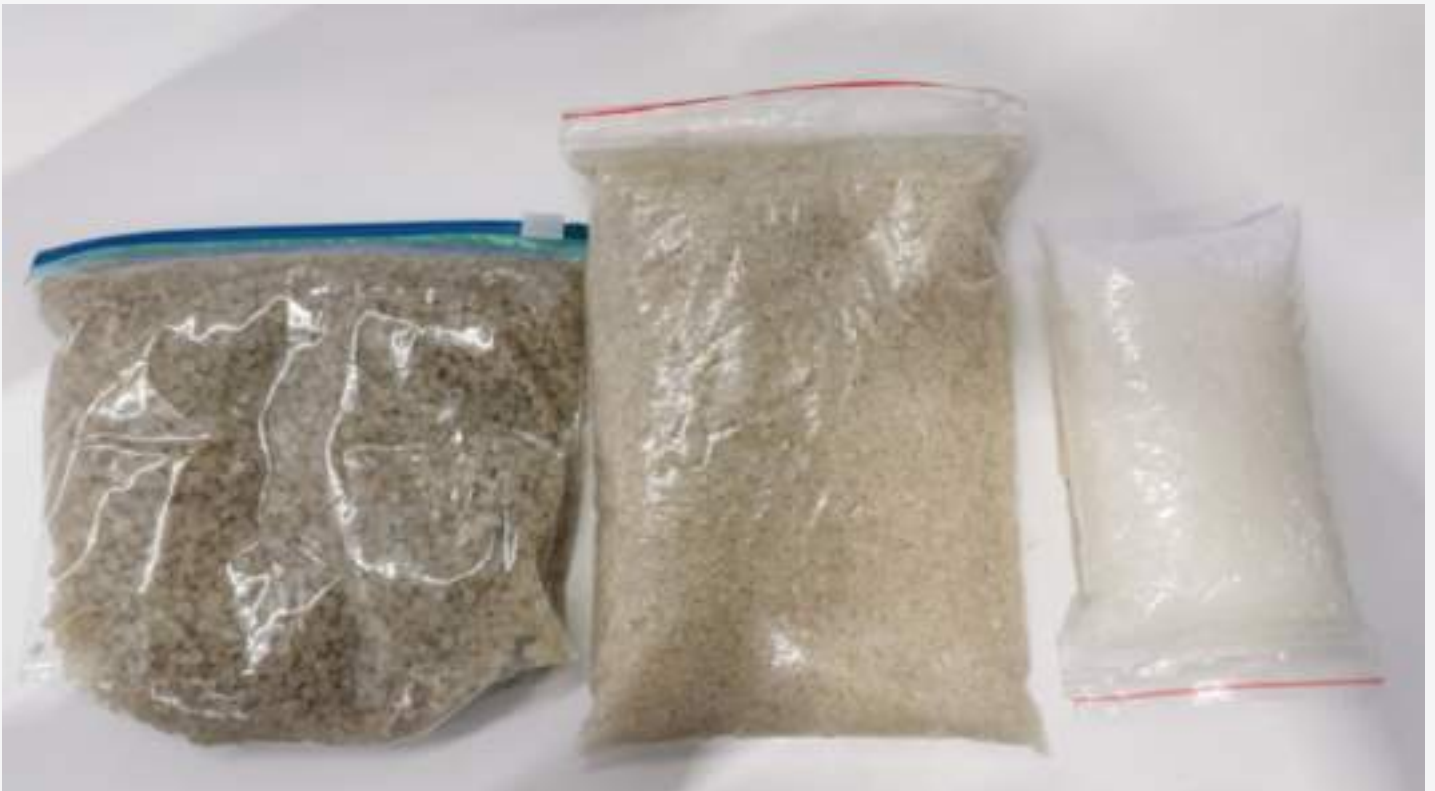
Figure 13. Different grades of recycled polyethylene (left and middle) compared to virgin polyethylene (photo by Roland Weber). ▼
